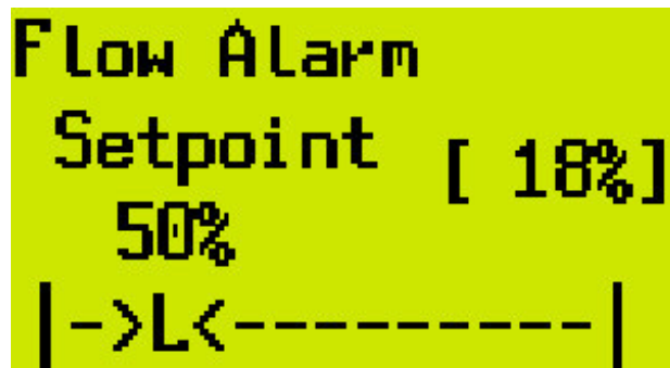
Figure 5. FLOW ALARM screen
