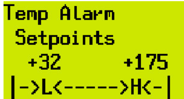
Figure 7. TEMPERATURE ALARM screen (w/ hi-temp setpoint)
